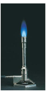
Methane reacts with oxygen to produce the flame in a Bunsen burner.
