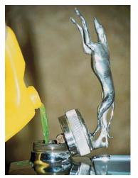
The addition of antifreeze lowers the freezing point of water in a car's radiator.
