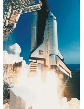
The main engines in the space shuttle Endeavour use hydrogen and oxygen as fuel.
