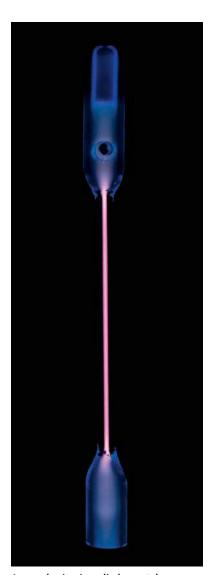
Argon glowing in a discharge tube.
