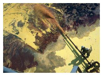
(left) A sulfur deposit. (right) Melted sulfur obtained from underground deposits by the Frasch process.
