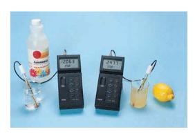
**FIGURE 14.9** pH meters are used to measure acidity.
