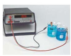
A concentration cell with 1.0 M Cu<sup>2+</sup> on the right and 0.010 M Cu<sup>2+</sup> on the left.
