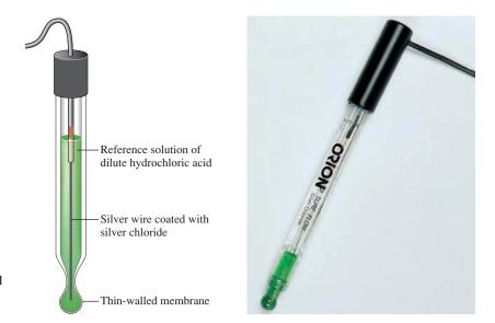
A glass electrode contains a reference solution of dilute hydrochloric acid in contact with a thin glass membrane in which a silver wire coated with silver chloride has been embedded. When the electrode is dipped into a solution containing H<sup>+</sup> ions, the electrode potential is determined by the difference in [H<sup>+</sup>] between the two solutions.
