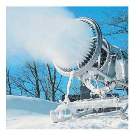
A snowmaking machine, in which water is blown through nozzles by compressed air. The mixture is cooled by expansion to form ice crystals of snow.
