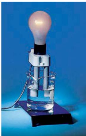
An acetic acid solution, which is a weak electrolyte, contains only a few ions and does not conduct as much current as a strong electrolyte. The bulb is only dimly lit.
